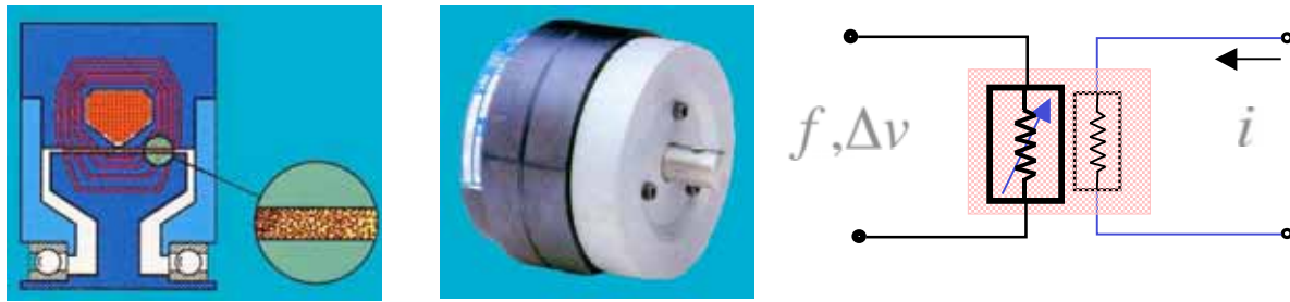
Figure 5.38 Magnetic powder controlled clutch. Electromechanic transducer schematic.
