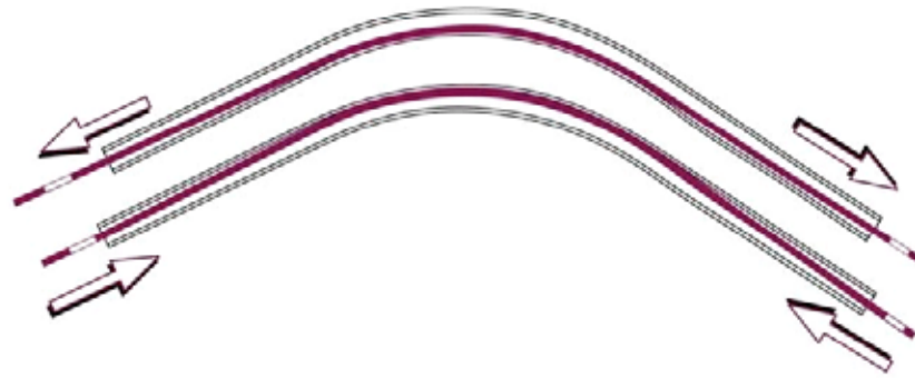
Figure 5.21: Backlash in push-pull systems
