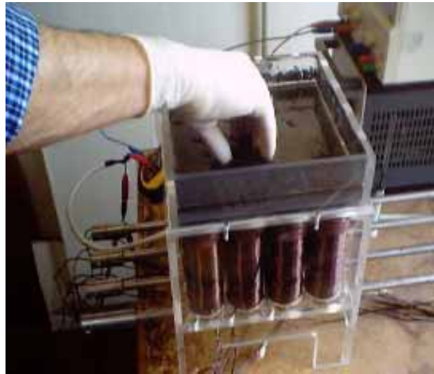
Figure 6.63 - Haptic Black Box composed of 16 vertical solenoids
